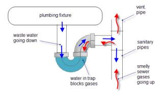
A p-trap is u-shaped plumbing device which prevents odorous gases in plumbing drains and sewers from rising up through toilets, sinks and floor drains.
